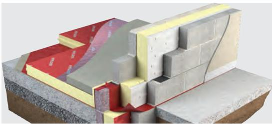
2. Where required, Radon barriers or DPCs should be dressed over the cavity either dissecting the board or dressed behind the riser boards and across the cavity below the insulation. The insulation should be butted tightly either side of the barrier to provide thermal continuity. Preformed detailing of radon barriers provides a more accurate solution. Contact the membrane manufacturer for further guidance on installation and best practice.
