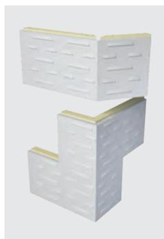
4. Install the first row of insulation boards, allowing for the floor insulation overlap, supported by at least 2 wall ties per board. Boards should be installed with the tongue upper most and the profiled face outer most, placed tightly against the inner face of the outer blockwork.
